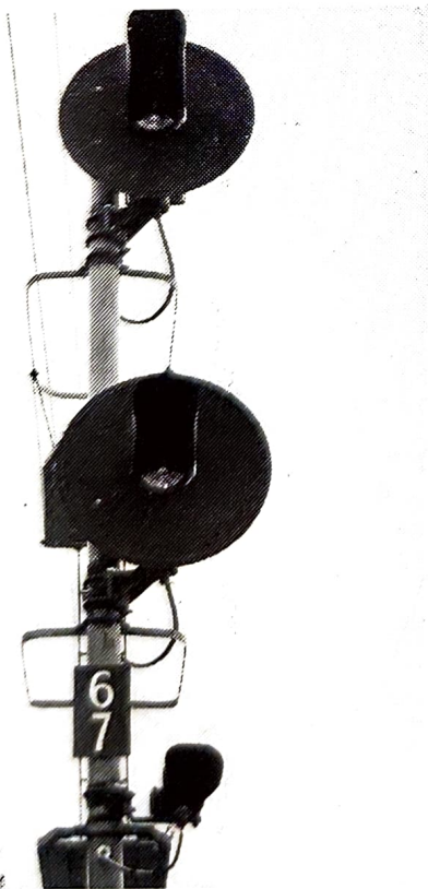
Three Position Light Signals
